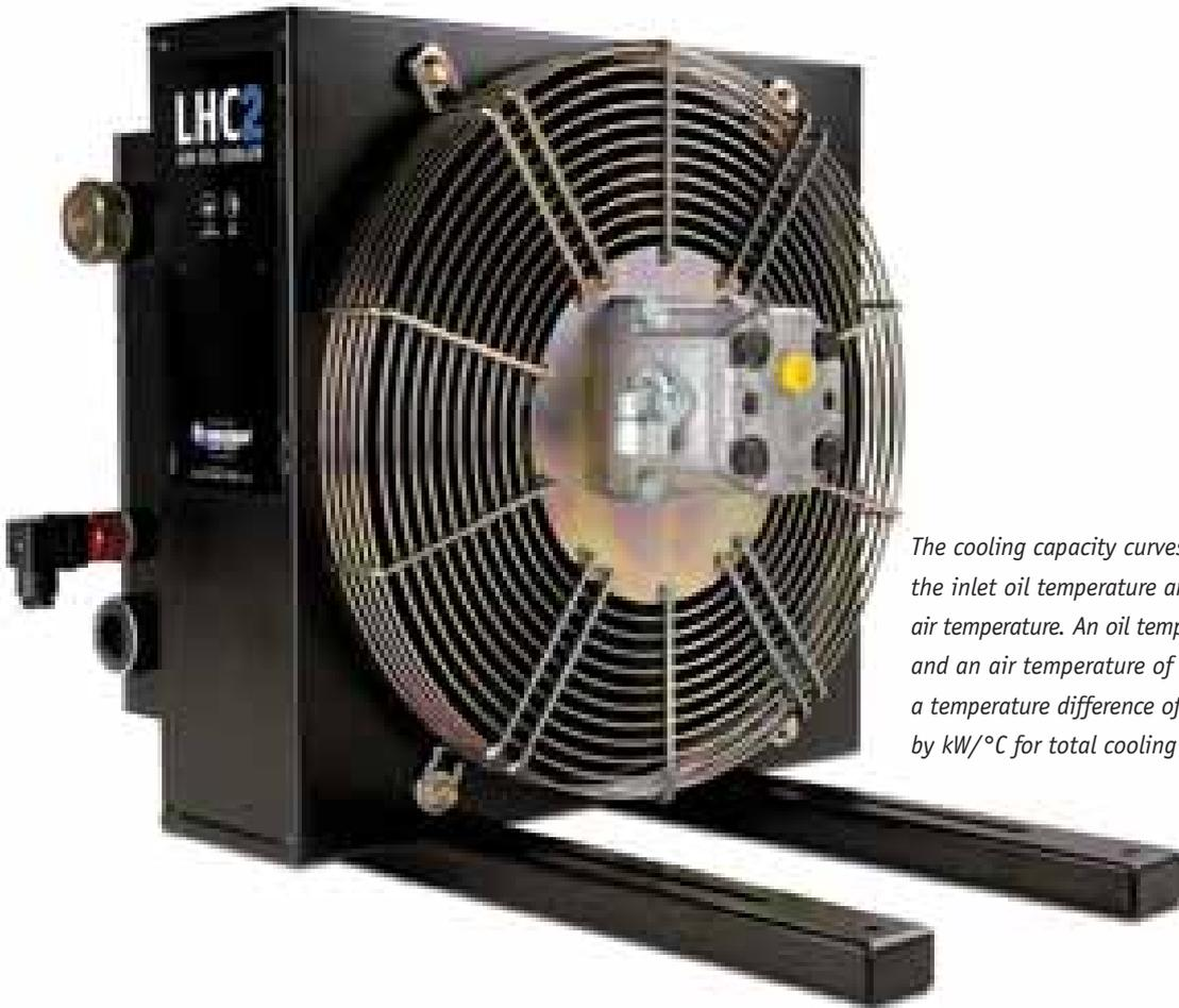
The cooling capacity curves are based on the inlet oil temperature and the ambient air temperature. An oil temperature of 60 °C and an air temperature of 20 °C produces a temperature difference of 40 °C. Multiply by kW/°C for total cooling capacity.
